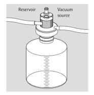
Place Sartolab 150v on the bottle neck. A vacuum is automatically created when used with a water jet pump or other vacuum source.
