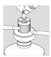
To fill multiple receiving bottles, break the vacuum with the valve on top of the Sartolab 150v housing.
