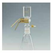
All areas, where liquid and device can get directly in contact, are made of glass or PTFE. The device, in combination with solvent-resistant, hydrophilic RC-membranes (type 184, see page 16), is therefore ideal for ultracleaning and degassing solvents and solvent mixtures for HPLC, GC and AA.
