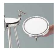
The major use of all three glass fibre filters is as a depth prefilter, placed directly on top of a membrane filter, whereby the prefilter diameter specified for the holder must be chosen. Larger diameters would intrude under the sealing ring of the holder and cause leakage.
