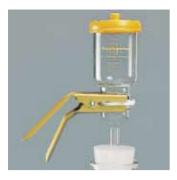
This filter holder is available in two versions differing from each other only in the type of the filter support. The filter with glass frit ensures uniform distribution of retained particles and is therefore recommended, when the residue on the filter surface is of interest. The device with PTFE-coated screen support, on the other hand, is due to its ease of clean more preferable, when the filtrate is required or when liquids difficult to remove from glass frits have to be examined.
