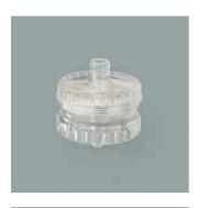
Polycarbonate holder for aqueous solutions This inexpensive filter holder is made of clear, autoclavable polycarbonate and offers a filtration area six times the amount of that of the 13 mm holder described on page 35. The silicone gasket enables a leak free filtration at pressures of up to 7 bar by simple, manual screwing together. Filter supports in the top and bottom parts allow filtration in either direction.
