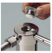
A practical holder for a lot of laboratory filtrations. It can be attached to a tripod with the help of a steel rod which can be screwed in. The hose nipple is screwed into the side of the top part in order to leave room for a large filling opening. This simplifies the pouring-in of the sample and the sample can be refilled without removing the tube connection to the pressure source. Leak-proof sealing is achieved by hand-tightening of the closing ring.
