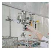
The inlet and outlet connectors are sanitary flanges, which are integral parts of the top and bottom plates. They assist in making the holder easy to clean and simplify the in-line installation. A suitable clamp allows, with the legs removed, to adjust the outlet at any height.
